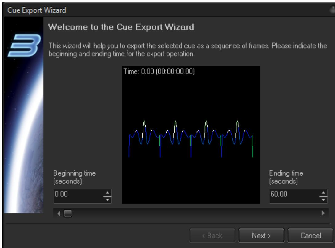
Once the Export Wizard is open, you will select the Beginning and Ending times to define the amount of the laser content image you want to export. BEYOND will calculate the number of frames to export based on the specified time range. The slider at bottom of the interface allows you to preview how the animation looks within the defined time range. Once the time range is set, click Next.
