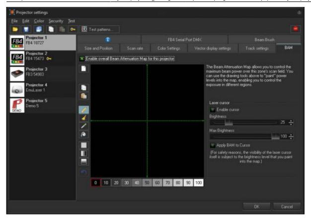
The **Beam Attenuation Map** allows you to control the brightness of a laser projector over the entire projection zone that it will correspond to, and it also allows non-uniform brightness maps. You can see a quick tutorial video about the BAM here: https://youtu.be/JQnQYPq5WzU?t=178
