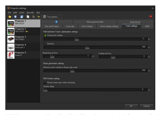
BEYOND generates special transitional (short) frames between the tracks/frames as well as between display updates. For example, if you display two cues, then BEYOND will inject a transitional path between them. The path is a blank line with a few anchor points in beginning and ending of the line.
