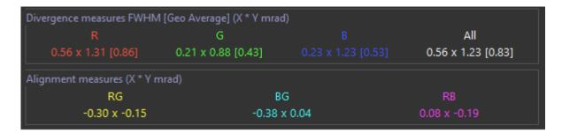
The LBA-C-100 is displaying the spot pattern as if it was projected at "infinity". To align the RGB and B or stacks of diodes, we should see 1 single spot on the LBA-C-100, with all colors superimposed.
