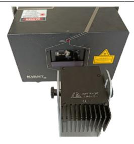
Place the LBA-C-100 in front of the laser output to measure, as shown in the following picture. Use the holder to adjust the height if necessary.
