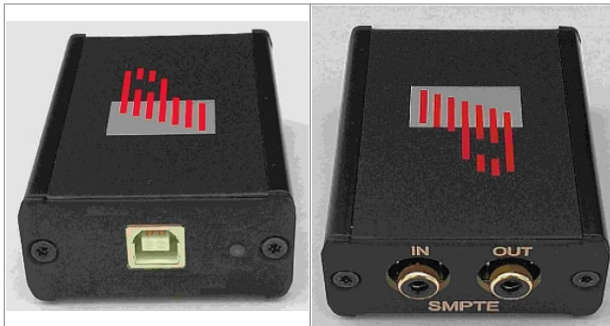
On one side we have a USB port, and an RGB status LED. On the other side we have RCA input and output for our Audio LTC, this is slightly different than the TC2000 as the TC2000 had 3 leds on the USB
