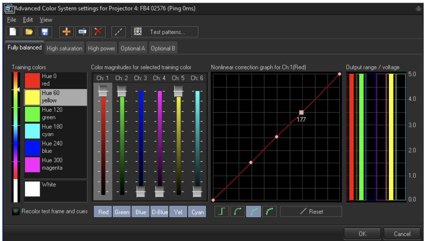
For Yellow training color BEYOND starts with 3 of the sliders in the 100% position. With an RGB projector, we make yellow out of green and red. That is why the Red and Green sliders are at 100%. However, if high end, the projector may have yellow laser, and the ILDA socket has a designated Yellow pin as well. That is why we also have Ch 5 (the Yellow Slider) at 100% too.
