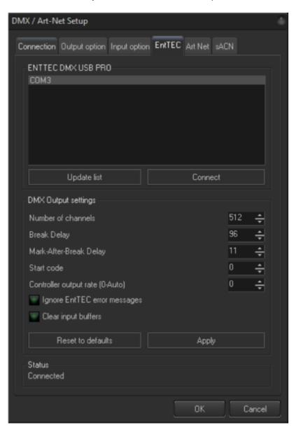
Before you can use a USB DMX Device with beyond, you must download and install the driver for that device to your PC. Once you have done that, BEYOND will recognize devices on COM Ports like the picture indicates. To connect, click on the com port, and click connect.
