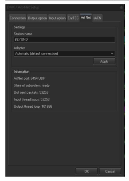
In this tab you can give BEYOND a station name to be recognized over the network and select the adapter you would like you're ArtNet to be sent and received on.
