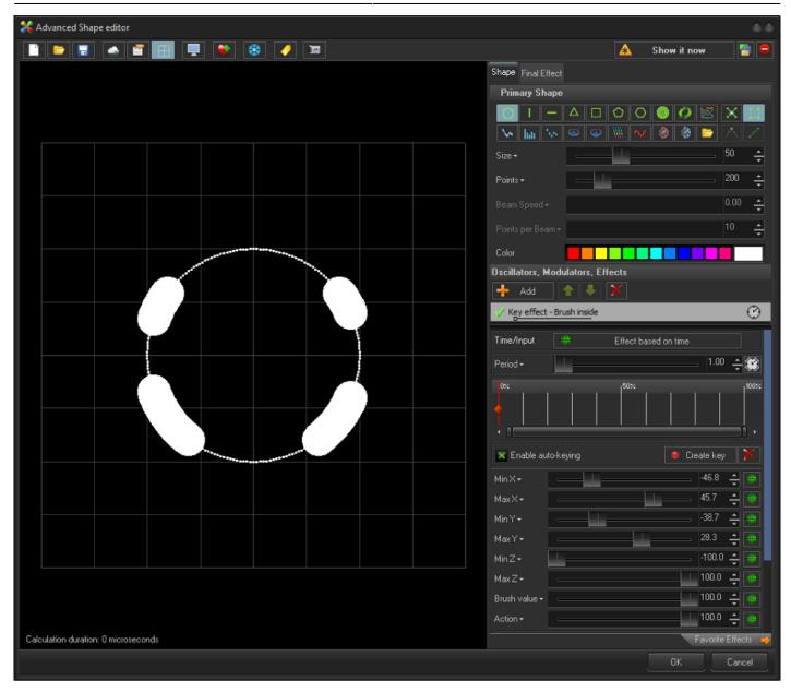
Just like window clipping and masking, we can change the brush value in inside the square shaped area determined by the minimum and maximum x axis and y axis. and you can set the brush value Inside that square.
