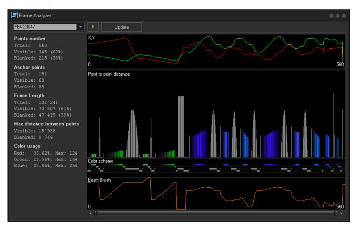
We have added Beam Brush® to this window to help you check the potential performance of your cue even if you do not have a Beam Brush® projector at your immediate disposal. The Beam Brush® device moves like an x or y scanner, so we represented it like so. It is always a good idea to check this to make sure your scanners and Beam Brush® will be able to handle what you are asking of it in the cue.
