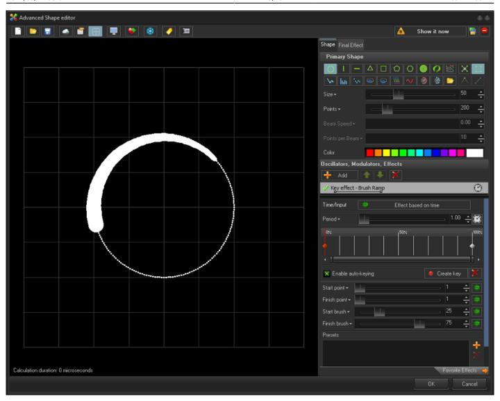
Brush ramp lets you set a start point of the frame, the end point of the frame, and ramp between a start brush value and end brush value this acts similar to how a color effect would modify points, but instead is done in a key effects to allow you animation between keys.
