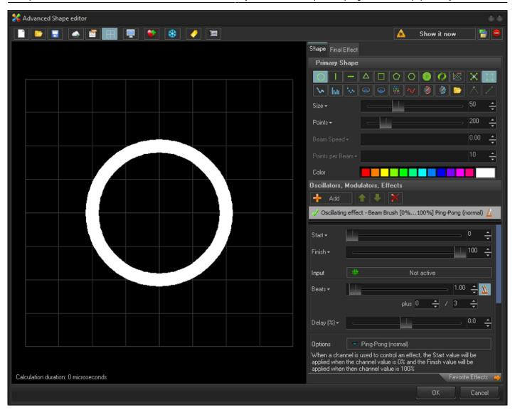
Beam Brush® (Oscillating effect type) will modify all points brush value. Using the start to finish values, you can animate between these values repeatedly over the time set in the beats, or seconds slider. You can also use the delay slider to change at what point the animation will start.
