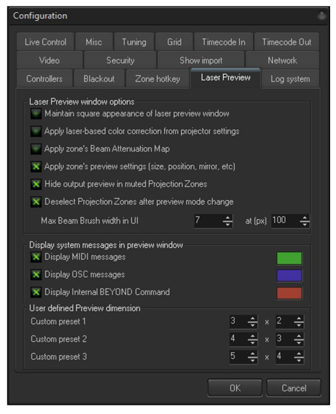
The laser preview will visualize Beam Brush® size. Use the "Max Brush Width in UI" to adjust the scale of brush in pixels. The default we recommend for most users is 7 at 100 pixels. You may need to increase
