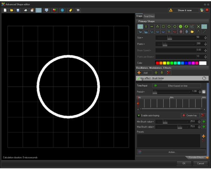
Brush limiter will change the minimum brush value of the frame, and maximum value of the frame. This can be used to change the brush value of an object without overriding previous brush effect values like color type brush effects. This modifies all points Inside the frame.
