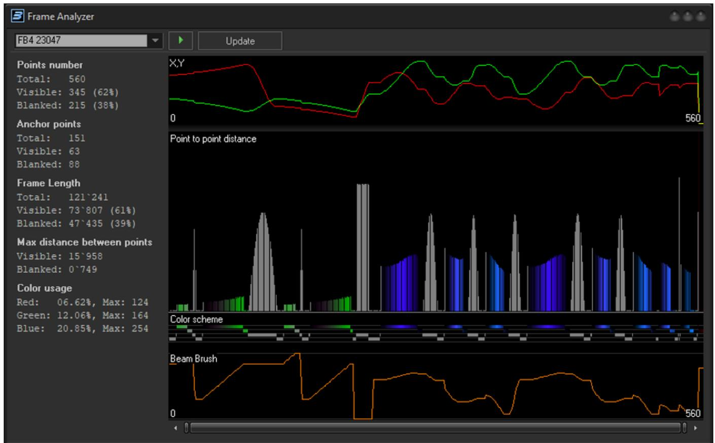
We have added Beam Brush® to this window to help you check the potential performance of your cue even if you do not have a Beam Brush® projector at your immediate disposal. The Beam Brush® device moves like an x or y scanner, so we represented it like so. It is always a good idea to check this to make sure your scanners and Beam Brush® will be able to handle what you are asking of it in the cue.
