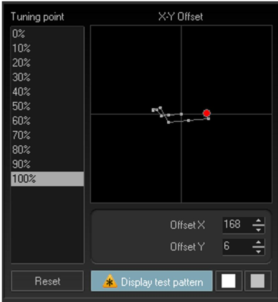
Beam Brush® systems as they move through brush values will create a slight X-Y shift in output. This can be minimized with perfect alignment, but in the reality of the touring world, this is unachievable, so we have added a X-Y compensation to tune this shift and make your output perfectly smooth. This X-Y offset is done before the output scaling and Linearity correction This means that it counts for the full 100% of the potential brush range. So, scaling afterwards will not affect X-Y Offset.
