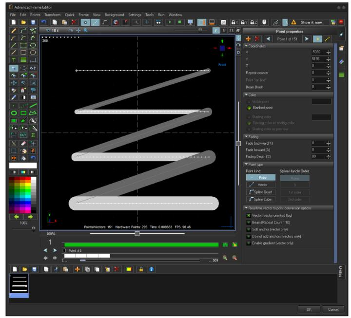
The advanced frame editor has added Beam Brush® features. On the left below the color selection you will see a slider, this is where you select the brush value you want to work with. This size will be applied to any new lines drawn while its selected.
