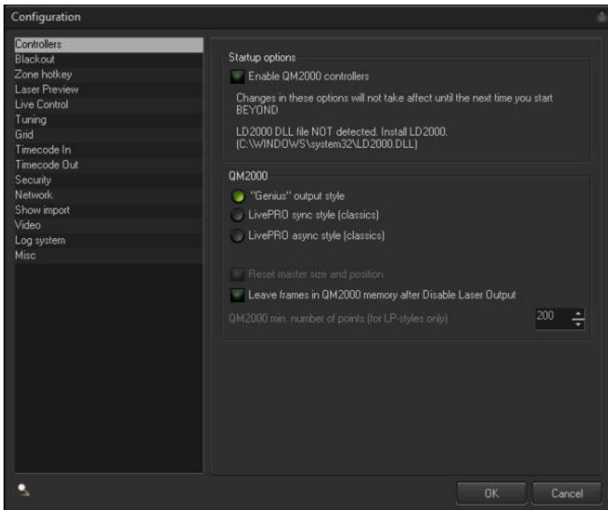
This setting will enable or disable the use of a QM2000. This is required when a PC has the LD2000 software installed, but no QM2000 hardware actually exists. **HINT: You can enable or disable the start of QM2000 controllers, during the startup of BEYOND. Right after BEYOND starts, hold the CTRL key. This will show the Welcome dialog option for the QM2000.**
