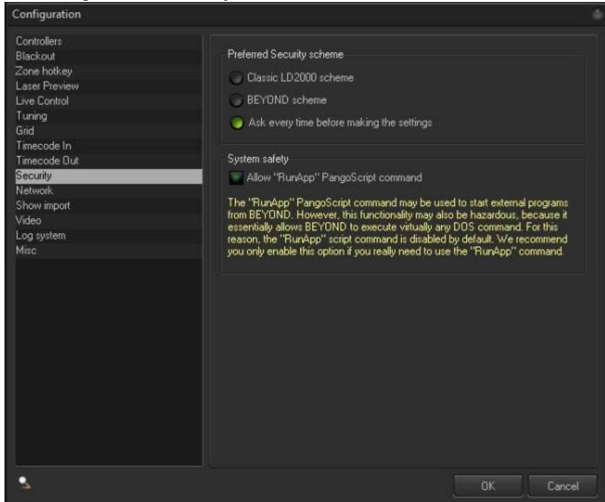
**“RunApp” PangoScript command - The RunApp command encapsulates the ShellExec() functions of the Windows, that can start programs, open documents and in some cases, do dangerous things. For safety reasons this command is disabled. Enable it only if you need to, and make sure you understand all of the risks associated before doing so.** ===== Network
