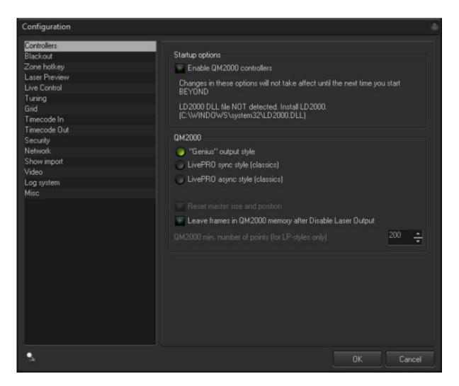
This setting will enable or disable the use of a QM2000. This is required when a PC has the LD2000 software installed, but no QM2000 hardware actually exists. **HINT: You can enable or disable the start of QM000 controllers, during the startup of BEYOND.** Right after **BEYOND starts, hold the CTRL key.** This will show the Welcome dialog option for the QM2000.
