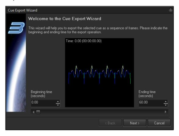
Once the Export Wizard is open, you will select the Beginning and Ending times to define the amount of the laser content image you want to export. BEYOND will calculate the number of frames to export bases on the specified time range. The slider at bottom of the interface allows you to preview how the animation looks within the defined time range. Once the time range is set, click Next.
