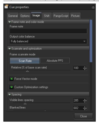
The **Image** tab has an embedded Image properties dialog that controls sample rate, vector settings, and a few additional parameters.
