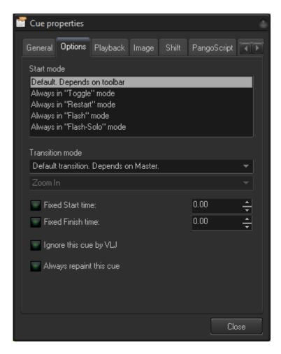
By default, the cue uses the click mode defined on the main toolbar - toggle, restart, flash. Start mode can assign modes to a cue permanently. For example, your situation may call for you to have some cues always in Flash mode, or some in Flash-Solo. Note: you can use two grids, and each grid has its own click mode.
