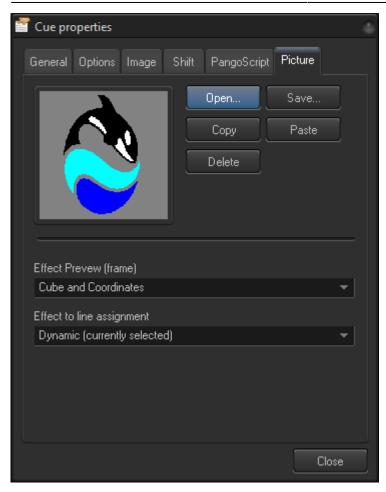
Cues may have a static picture as a background of the cue. There are file operation buttons, **Open** and **Save, Copy** and **Paste** for Clipboard and a Delete button to delete the picture.
