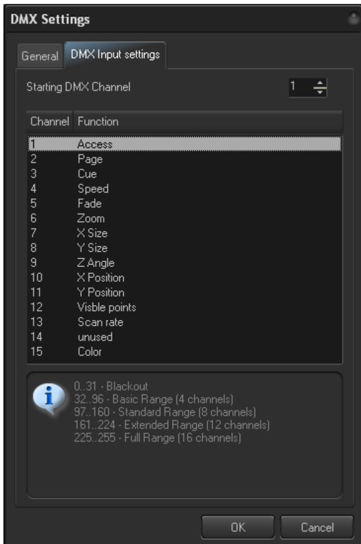
As shown above, the DMX Channel Assignment for BEYOND is exactly the same as that of the FB3-SE DMX daughter board. This allows external controllers that are already familiar with the FB3 to easily control BEYOND in the same way and providing the same results.
