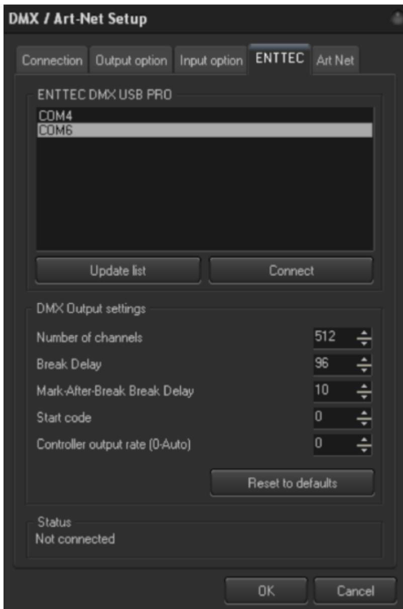
If you have the proper COM port selected, and the device is connected and working properly, BEYOND should produce a pop up message that will show the serial number and firmware version installed in the device, as shown above.
