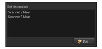
**Set Zone** - removes routing information of incoming laser content and redefines the routing based on its own settings. This is simple redirection.
