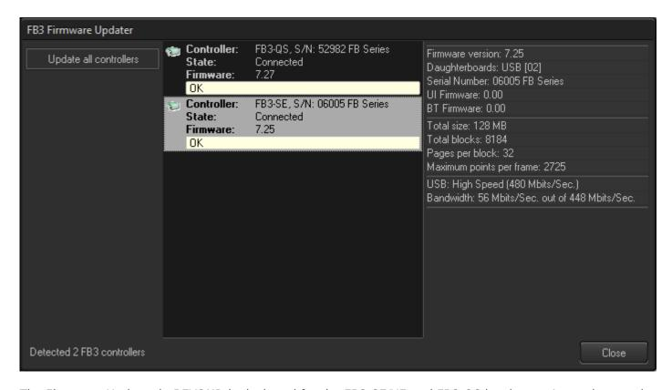
The Firmware Updater in BEYOND is designed for the FB3-SE/XE and FB3-QS hardware. As a rule, you do not need to worry about the firmware version of your hardware because BEYOND checks the firmware version when it opens or an additional hardware controller is connected to the system (while BEYOND is open) and updates the firmware automatically. The firmware is embedded into BEYOND; you do not need to browse your computer to select files of do anything else.
