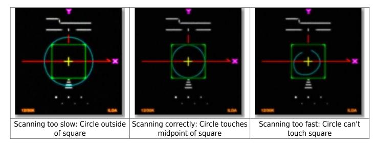
As you are projecting the ILDA test Pattern, look very carefully at the central section of the test pattern. Adjust the Default Scan rate slider in the Projector Settings window so that the circle is just touching the sides of the square. Note that sometimes the circle may touch only the sides but may be over on the top and bottom, or vice versa. Just adjust the slider for the best overall appearance of circle touching the square.
