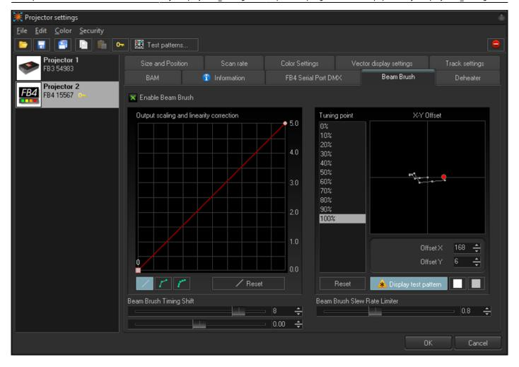
**Output Scaling and Linearity Correction**
