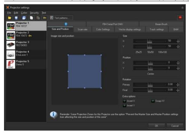
Size and Position are "global" settings of the Projector. "Global" means all Projection zones that go to this Projector will be influenced by this setting. The Projection Zone menu has Geometric correction settings which can appear to create some redundancy.
