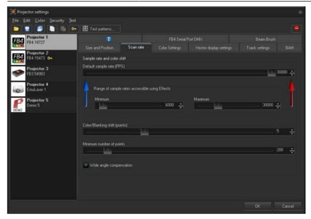
**Default sample rate** values should be tuned using Test patterns. There is direct relation between default sample rate, color shift, Sample rate, Size, and Position. Bigger size means a larger angle and as a result more time is required for motion; your Sample rate should be lower. Conversely, for smaller angles, the sample rate can be higher.
