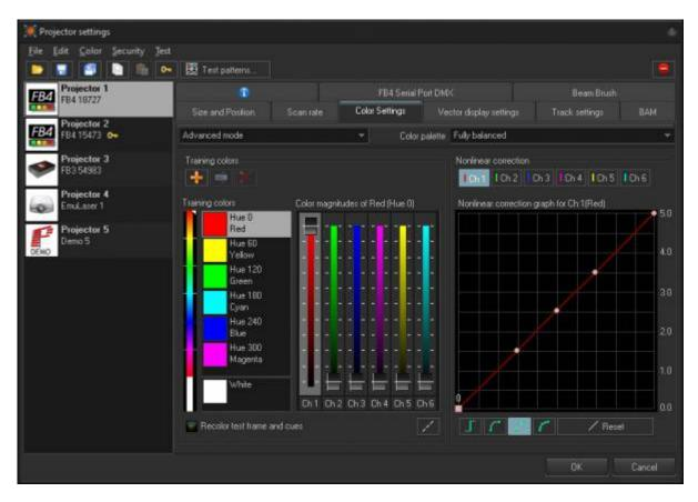
The Advanced mode allows for 6 color channel setup. Its important to note that if your laser has more then RGB inside, you will need to go to Advanced mode to actually use the extra color channels.
