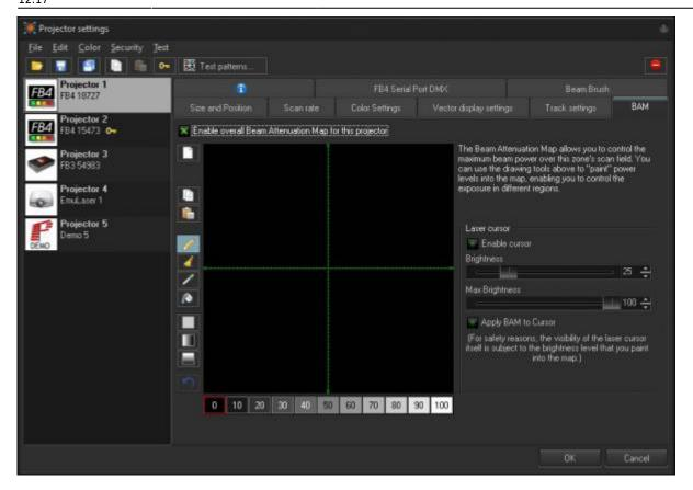
The **Beam Attenuation Map** allows you to control the brightness of a laser projector over the entire projection zone that it will correspond to, and it also allows non-uniform brightness maps. You can see a quick tutorial video about the BAM here: https://www.youtube.com/watch?v=89xLGkicUjl
