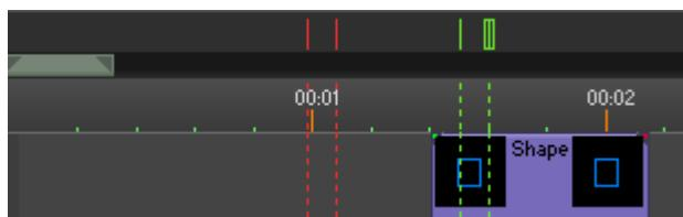
Time markers are very important if you want to work quickly within a TimeLine show. They have multiple actions that are used to create a visual indication of important places on the TimeLine. Lines work as a “snap-to” lines. When you edit an Event’s start or end position, the event will snap to the marker.
