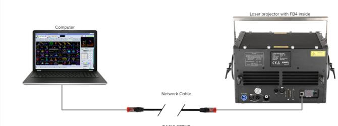
**BASIC SETUP**In this setup we have a single laser projector connected to our PC via the Integrated FB4 hardware.
