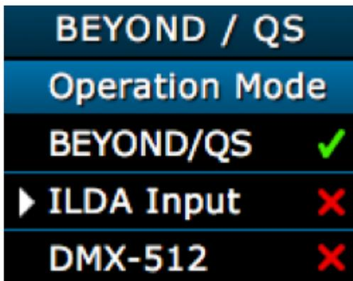
Push the button once. The new operation mode (ILDA input) is now active.
