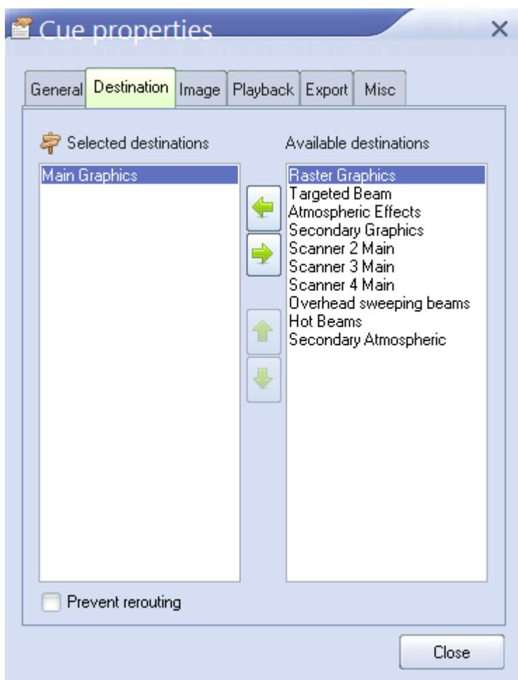
The **Destination** tab controls the destination of the cue (i.e. where the cue will be routed once it is triggered). Note that you can specify that the cue be directed to more than one zone (i.e. laser) simultaneously, so if you check both the “Zone 1” and “Zone 2” boxes above, the cue will be directed to both lasers simultaneously.
