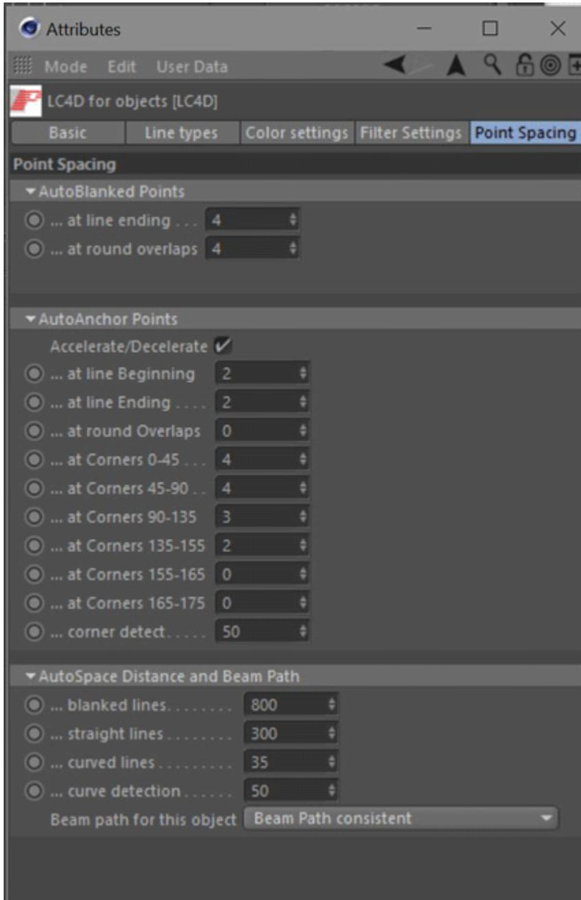
**Note:** The numbers shown above are the default values. They are optimized for scanners tuned to the ILDA 30K standard, when running at a point output speed of 30,000 points per second. If you do not change any of the numbers, objects will use the default values. For more information, see the topic [Scan speeds and LC 4D](#).
