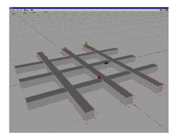
The height, width and length of the cross beams were decreased ever so slightly. This allows the renderer to determine that the surfaces of the blue beams is on top of the surfaces of the other beams.
