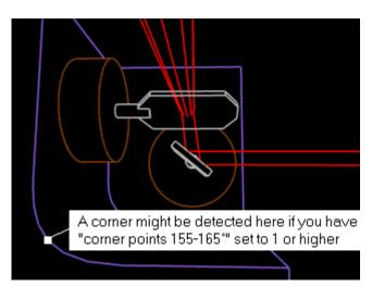
But what if there were instances where you wanted extra corner points at angles between 155 and 165 degrees? In this case, you can tell Lasershow Converter 4D that you still want corner points at these angles, but reduce the corner detection sensitivity by setting **Corner detect** to a lower value such as 10.
