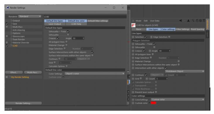
As you can see in the Lasershow Converter 4D object tag settings, the transparency, backfaces, and the prevent laser output option are disabled. For the selection we chose 10 contour lines in object y direction
