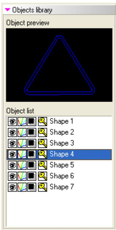
The Object Library has two purposes. First, it allows you to select and preview each object in the FLASH file. Second, it allows you to control various aspects of the rendering and laser output.
