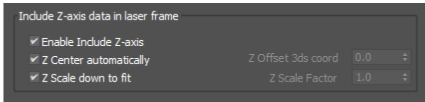
As a non-photorealistic renderer, Lasershow Converter MAX typically creates only two-dimensional output in the laser frames. That is, the laser frames have only X and Y data that change, and normally the Z-axis data is set to zero. However, for certain special effect applications, it may be handy to have the plugin include Z-axis data.
