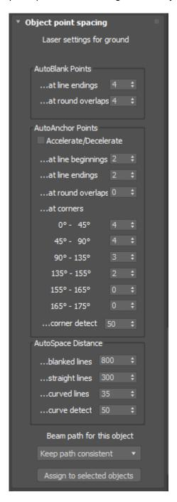
**Note**: The numbers shown above are the default values. They are optimized for scanners tuned to the ILDA 30K standard, when running at a point output speed of 30,000 points per second. If you do not change any of the numbers, objects will use the default values. For more information, see the topic Scan speeds and LC MAX.
