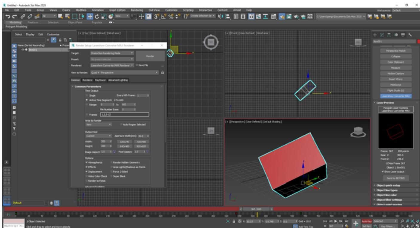
Just below the preview window in the utility plugin, you will see a check box called **Show Laser Output**. When this is checked, laser output will be shown on the laser projector in real time.
