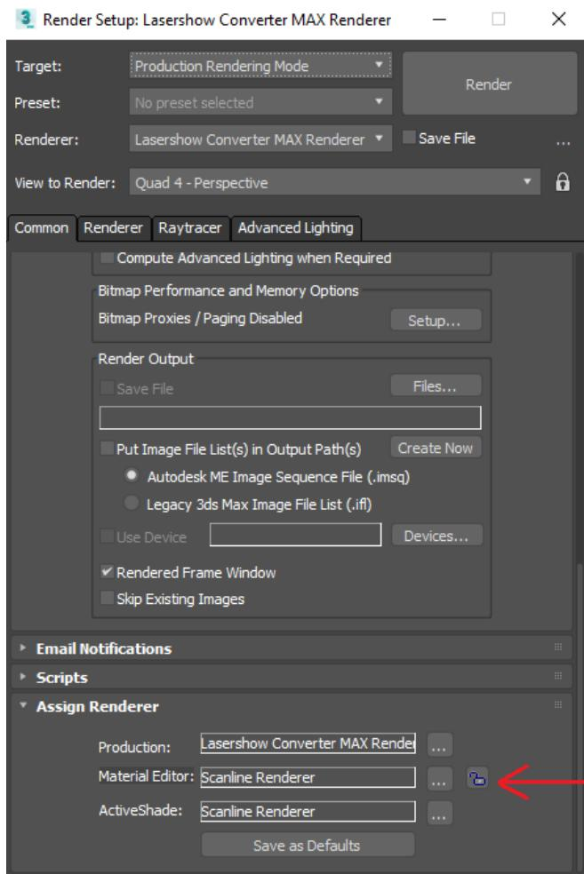
**Note:** Lasershow Converter MAX can not be used as the **ActiveShade** renderer.
