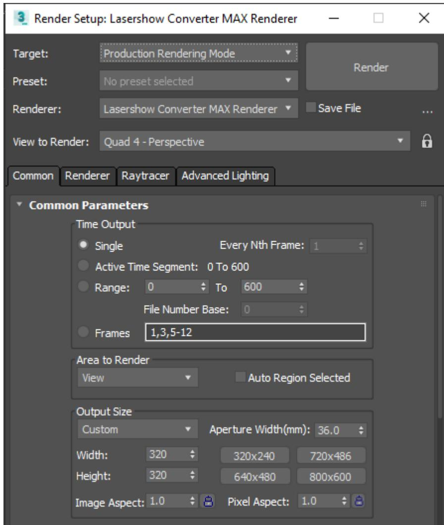
**Note:** Lasershow Converter MAX does filtering calculations, corner detection calculations and curve detection calculations based on the **Output Size** settings. The default values for the filter, curve and corner settings are based on a frame window output size of 320-by-320 or 320-by-240. If you choose a different output size (such as 640-by-480), this may require you to change Lasershow Converter MAX's filter, corner and curve settings.
