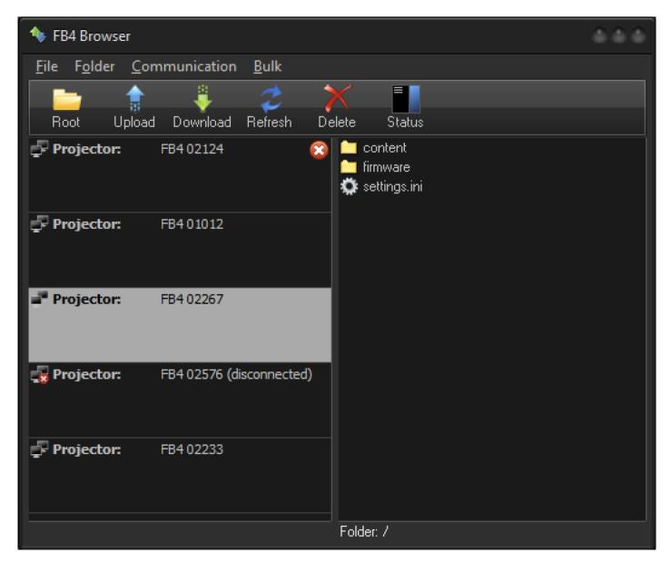
The FB4 needs to be connected to BEYOND/QS software to enable operations with the SD card. The left side of the window shows a list of connected FB4 hardware. The list indicates the Projector serial or name, connection state, presence of errors and the upload/download progress (if there are active operations).
