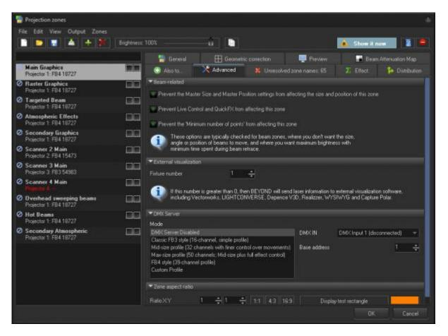
When the **Prevent master size and master position** check box is checked, it will make it so that the Master Size and Master Position controls in the **Projector Settings** window do not affect the output of this zone.
