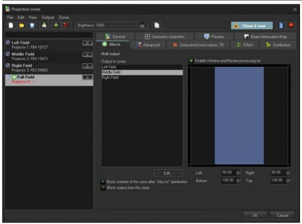
BEYOND calculates the output for each projector independently. This means that each projector has its own time, and the core calculates the frames of time for each projector. This time difference is not visible on a short frame, but it becomes very noticeable on long frames. Window clipping is not a solution for the display of really complex graphics. Results depends on the content.
