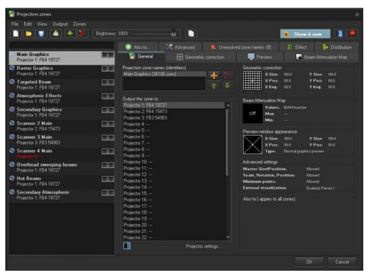
The list of projection zones can be seen and selected on the left side of the window. When you click on a zone on the left side, the tabs on the right allow you to view and adjust the parameters for each projection zone. To view and adjust the parameters, click on the **Geometric Correction, Preview Window Appearance, Beam Attenuation Map, Also to, Effect, or Advanced tab.**
