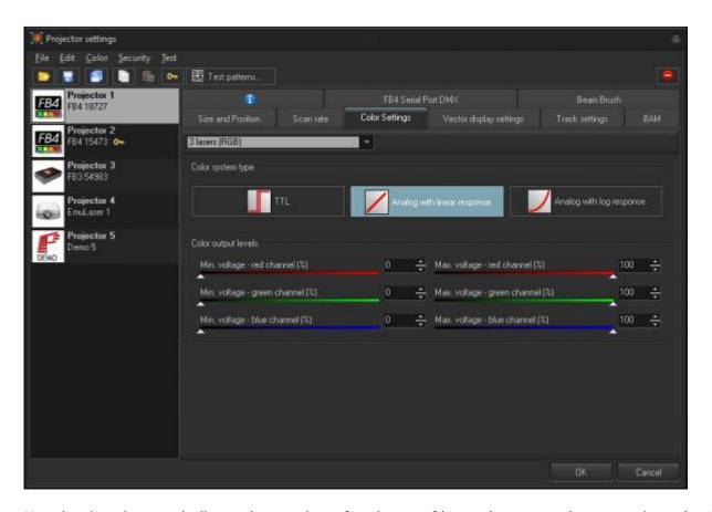
Use the dropdown to indicate the number of and type of lasers in your projector, and set the "color system type" using either TTL, Analog with linear responce or analog with log responce. Most users should use linear, or log for better low brightess resolution. BEYOND offers a few standard modes for quick setup and an Advanced mode that provides more flexible options.
