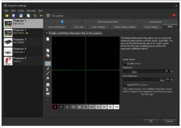
The **Beam Attenuation Map** allows you to control the brightness of a laser projector over the entire projection zone that it will correspond to, and it also allows non-uniform brightness maps. You can see a quick tutorial video about the BAM here: https://www.youtube.com/watch?v=89xLGkicUjI
