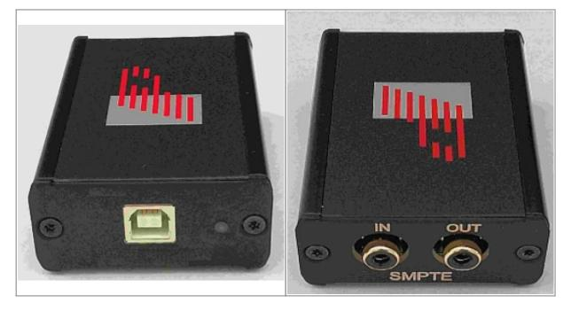
On one side we have a USB port, and an RGB status LED, On the other side we have RCA input and output for our Audio LTC, this is slightly different then the TC2000 as the TC2000 had 3 leds on the USB
