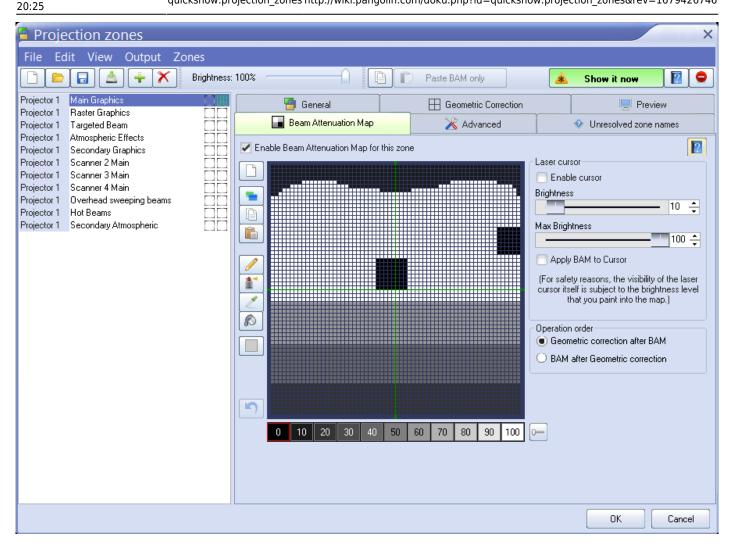
The **Beam Attenuation Map** is a 64 by 64 "pixel" brightness control map. Each pixel can be set to any brightness level from 0 to 100%. Rudimentary tools are provided to sample a brightness level in the map, fill the entire map with the selected brightness level, fill a rectangular area with the selected brightness level and freehand-draw brightness levels into the map.
