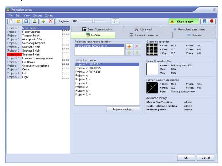
There are 30 projection zones which can be selected on the left side of the window. When you click on a zone in the left side, the tabs on the right allow you to view and adjust the parameters for each projection zone. To view and adjust the parameters, click on the **Geometric Correction, Preview, Beam Attenuation Map** or **Advanced** tab.
