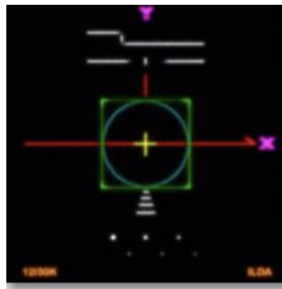
Color shift correct: Horizontal lines approximately centered
