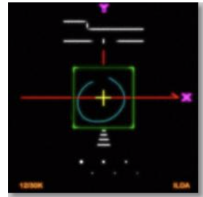
Scanning too fast: Circle can't touch square
