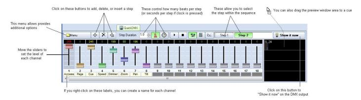
The main features of the **QuickTargets** tool are shown and described in the picture below.
