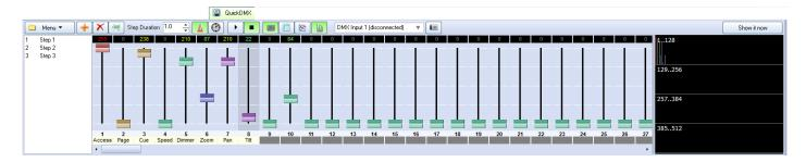
As shown, you simply add as many steps as you want in the sequence, moving the sliders at each step, indicate the step duration, and then either **Show it now**, or drag and drop the sequence to a cue for playback later.
