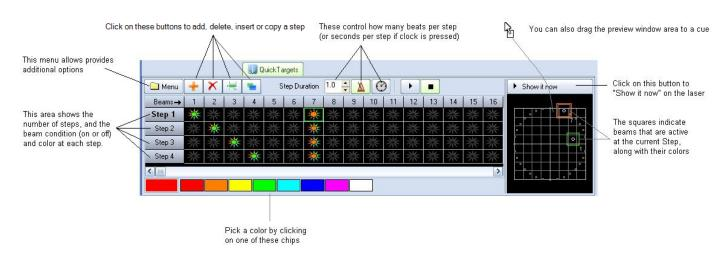
The main features of the **QuickTargets** tool are shown and described in the picture below.
