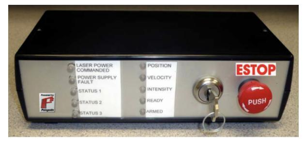
PASS may be controlled by, and may illuminate LEDs on an external control panel that is connected to PASS. Below is a description of the control panel connections. When PASS is not connected to an external control panel, then PASS will automatically reset into a "ready" state shortly after power up. When PASS is connected to an external control panel, then PASS will not power up in a "ready" state and instead, will wait for the "Manual Reset" from the control panel.
