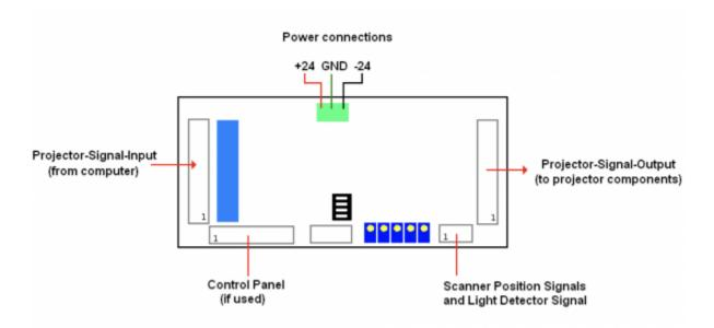
The general layout of PASS is shown above, with connectors identified.
