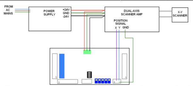
If you are using a one dual-axis scanner amplifier, the recommended connections are shown below:
