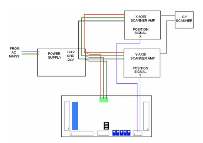
PASS monitors the power supplies that feed the scanner amplifiers. This voltage can be between  $\pm$ 0 volts and  $\pm$ 1 volts. The manor in which you connect PASS to the power supply and to the scanner amplifiers depends heavily upon whether you are using two separate single-axis scanner amplifiers, or
