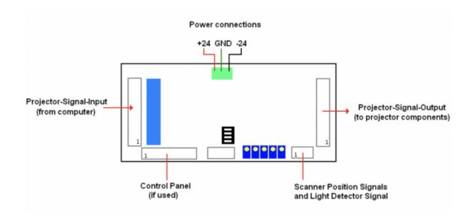
The general layout of PASS is shown above, with connectors identified.
