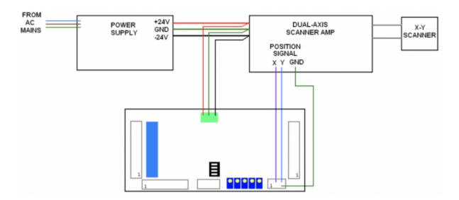
If you are using a one dual-axis scanner amplifier, the recommended connections are shown below:
