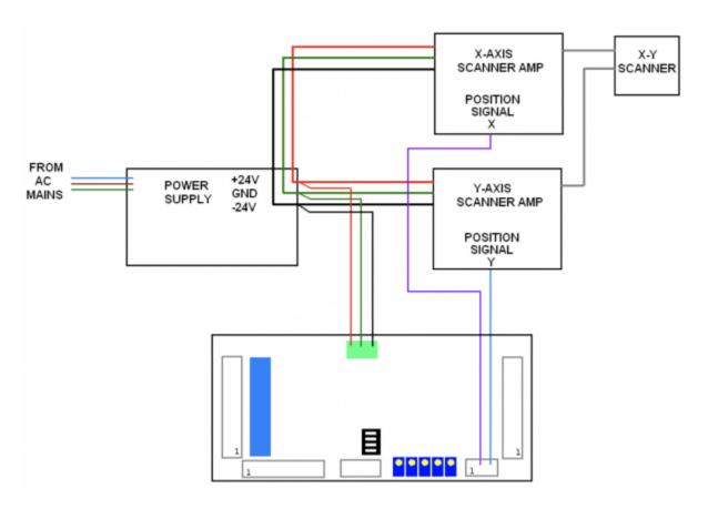
PASS monitors the power supplies that feed the scanner amplifiers. This voltage can be between  $\pm$ 0 volts and  $\pm$ 1 volts. The manor in which you connect PASS to the power supply and to the scanner amplifiers depends heavily upon whether you are using two separate single-axis scanner amplifiers, or one dual-axis scanner amplifier.
