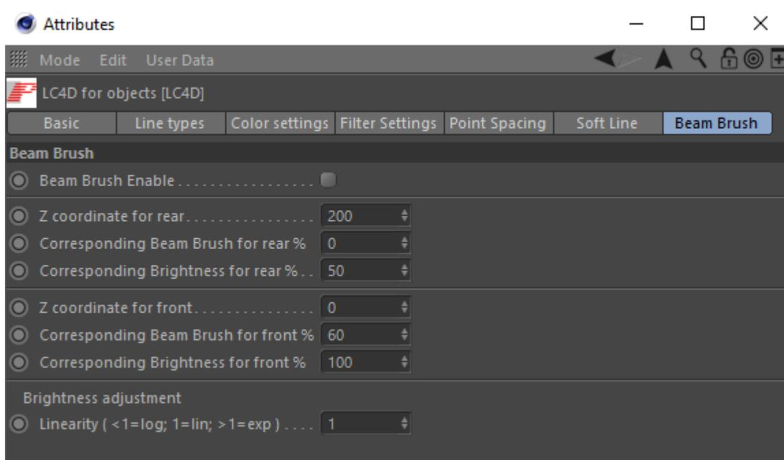
Beam Brush is dynamic beam divergence technology manufactured by the ScannerMAX division of Pangolin, and included in certain projectors manufactured by Kvant. The Beam Brush features of the Lasershow Converter MAX plug-in allow you to effectively map the Z-axis coordinate data from 3ds Max onto the beam diameter found in the 3ds Max objects. Each object can have its own Beam Brush settings, providing tremendous power and flexibility.
