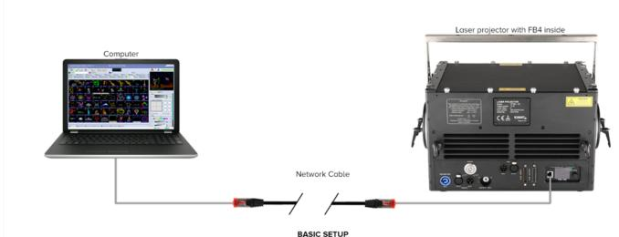
In this setup we have a single laser projector connected to our PC via the Integrated FB4 hardware.
