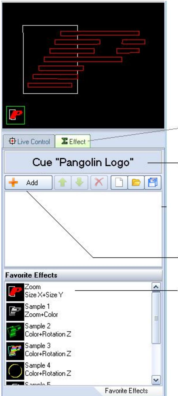
The Effect Editor is continuously available, and can be found on the right side of the QuickShow window, below the Preview window and on the right side of the Live Control tab
