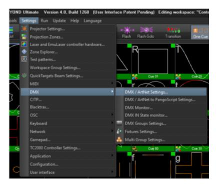
DMX (along with other 512 protocols) can be setup here, including USB DMX Devices like ENTTECH USB DMX PRO devices, Streaming Data through serial port on FB4, the DMX input and output on the OM2000.net, and over the network with Art Net and sACN.
